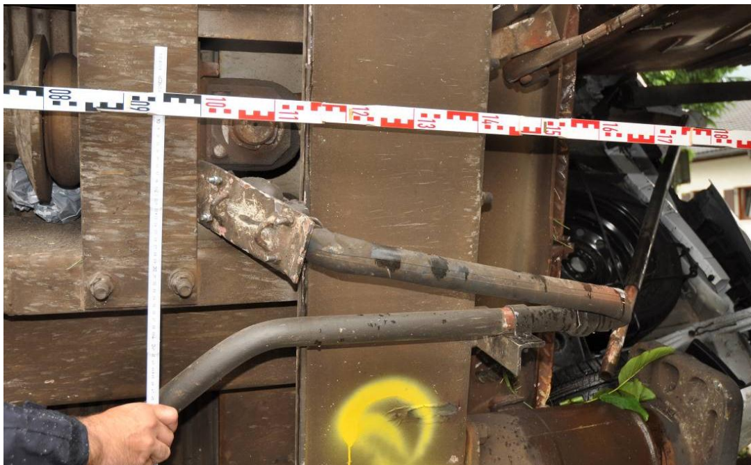
Figure 16 Kinked air hose with brake coupling (source: Bregenz CID)
