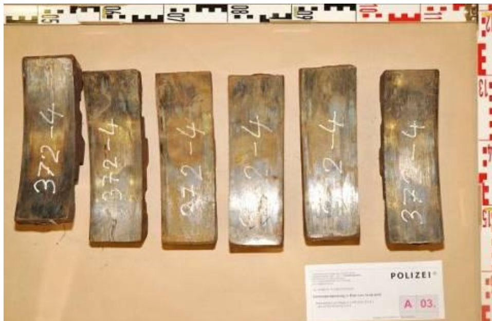
Figure 37 Brake blocks from the following section of the wagon (source: Bregenz Criminal Investigation Department)
