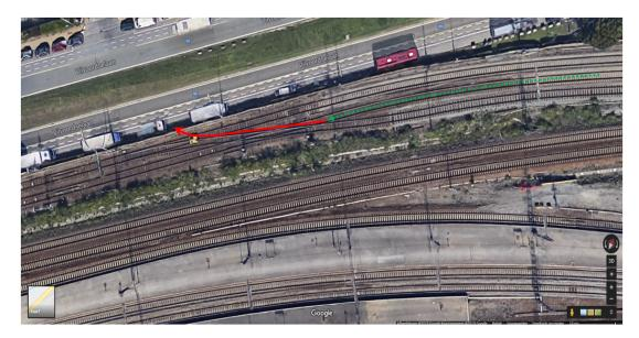
Locomotive HLE1312 derails at the end of the curve, damages the switch, crosses the adjacent track, and comes to a stop on the public road, where the locomotive collides with parked road vehicles. The first 3 wagons partially derail. During the derailment, the train driver is seriously injured.
