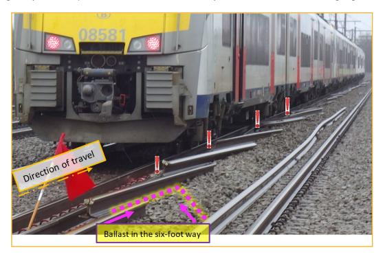
At the level of the first bogie of the train, the first damage to an axle-bearing can be observed. Later, when inspecting the rolling stock during the technical investigation, a piece of rail can be used to simulate that the course of the fracture line of the axle-bearing corresponds to the profile of the running surface.
