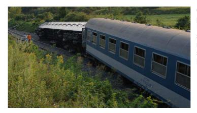
On 2 August 2008, 4 carriages of a passenger train derailed between Kurd and Szakály-Hőgyész stations, one of which toppled to its side. The rail track sustained substantial damage on a 200 metre length.
