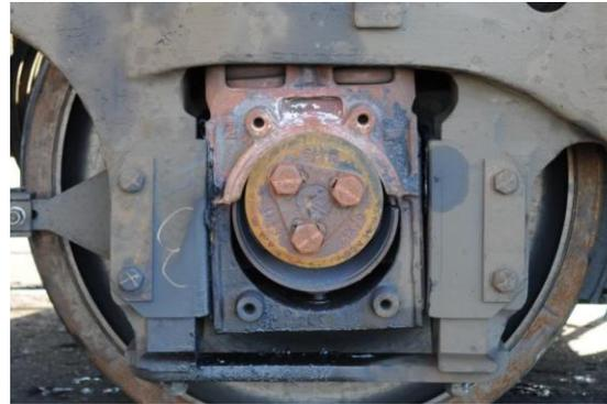
Figure 2 - Failed bearing in axlebox
