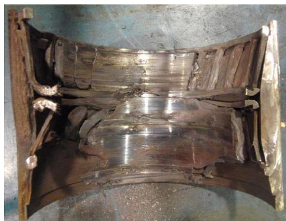
Figure 7 - Bearing cup raceways
