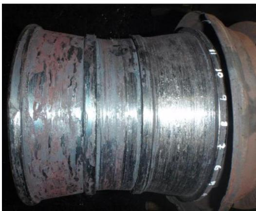
Figure 6 - Bearing cone raceways
