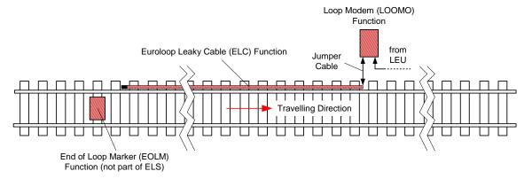
Figure 6-2: Possible Realisation of a Single Euroloop Arrangement
