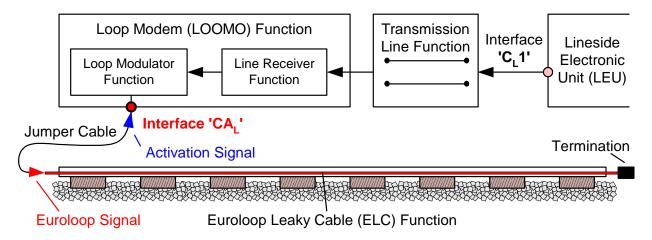
Figure 6-11: Signal Transmission between LOOMO and ELC
