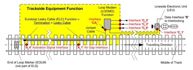
Figure 6-1: Trackside Equipment of Euroloop Subsystem (unidirectional installation)
