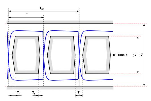
Figure 6-7: Transmit Pulse Shape Measured into a Resistive 120  $\Omega$  Load
