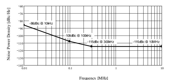
Figure 6-15: Single Sideband (SSB) Phase Noise of the Raw Carrier
