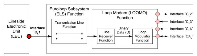
Figure 6-5: Data Transmission between LEU and LOOMO
