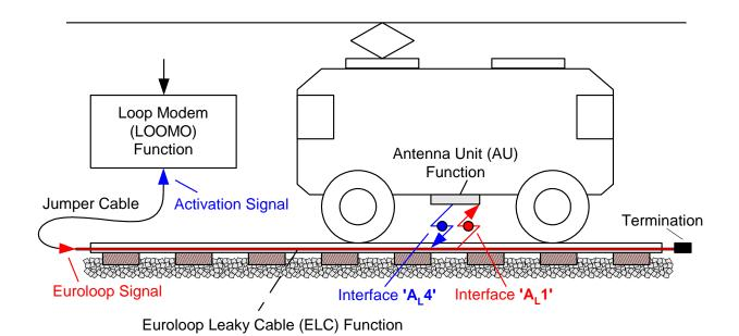
Figure 6-18: Air Gap Interfaces 'A<sub>L</sub>4' and 'A<sub>L</sub>1'
