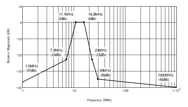
Figure 6-17: Spectrum Mask of Euroloop Up-link Signal
