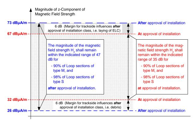
Figure 6-20: Limits of Magnitude of z-Component | H<sub>z</sub>| of Magnetic Field Strength H with Margins for Trackside Installations
