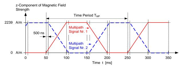
Figure 7-6: Time-Varying Multipath Signals
