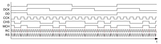
Figure 6-13: Signals Associated with DSSS Modulation (Informative)
