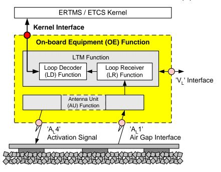
Figure 7-4: Kernel Interface of On-board Equipment
