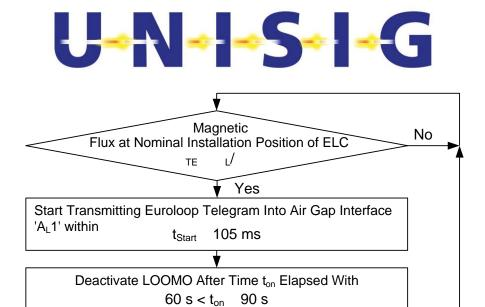
Figure 6-19: Flow Diagram for Activation of LOOMO by Activation Signal from Interface 'AL4'
