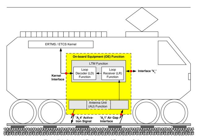
Figure 7-1: On-board Equipment of Euroloop Subsystem
