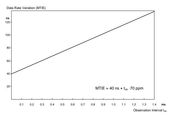
Figure 6-14: MTIE of the Modulation Signal
