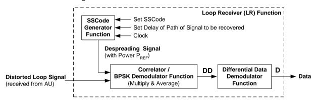
Figure B- 2:Functions Associated with Demodulation
