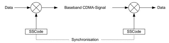
Figure B- 1: CDMA Modulator and Demodulator
