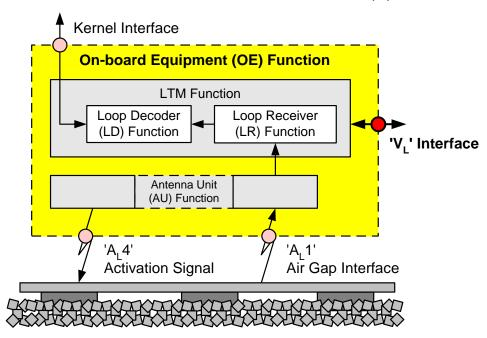
Figure 7-5: Interface 'VL' of On-board Equipment
