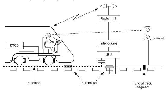
Figure 5-1: ERTMS/ETCS Level 1 with In-fill
