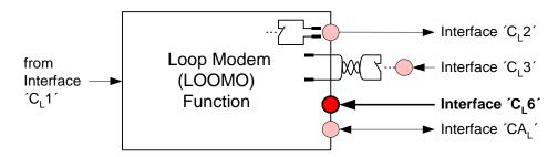
Figure 6-10: External Power Source Interface 'C<sub>L</sub>6' of LOOMO
