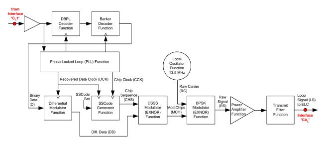
Figure 6-12: Principles of DSSS Modulator: Functions Associated with Modulation (Informative)
