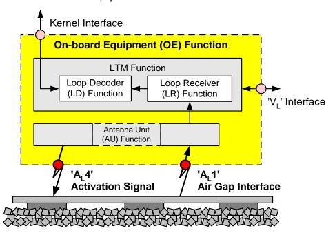
Figure 7-2: Air Gap Interfaces of On-board Equipment
