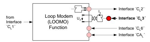
Figure 6-9: External Activation Interface 'C<sub>L</sub>3' of LOOMO
