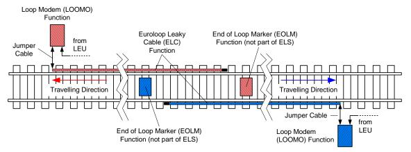
Figure 6-3: Possible Realisation of a Double Euroloop Arrangement
