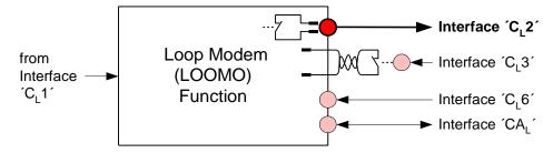
Figure 6-8: Error Indication Interface 'C<sub>L</sub>2' of LOOMO
