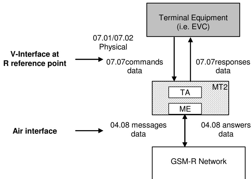
**Figure A1 : Interface between on-board Terminal and MT2 mobile Terminal**
