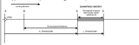
The minimum distance (latest transmission) between announcement of track condition Change of Traction System and the location of this track condition shall correspond to 17s when running at line speed (engineered SSP) in the approach area (B-F in the figure below).
