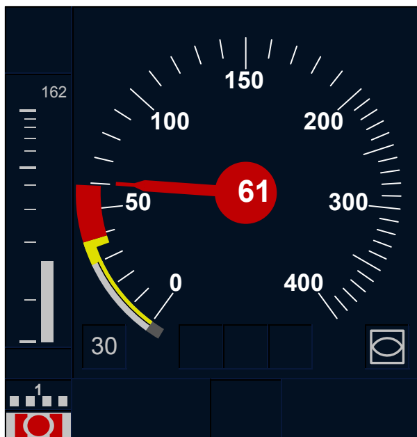
Figure 24 – Speed and supervision information in TSM / IntS (bubble 2++)
