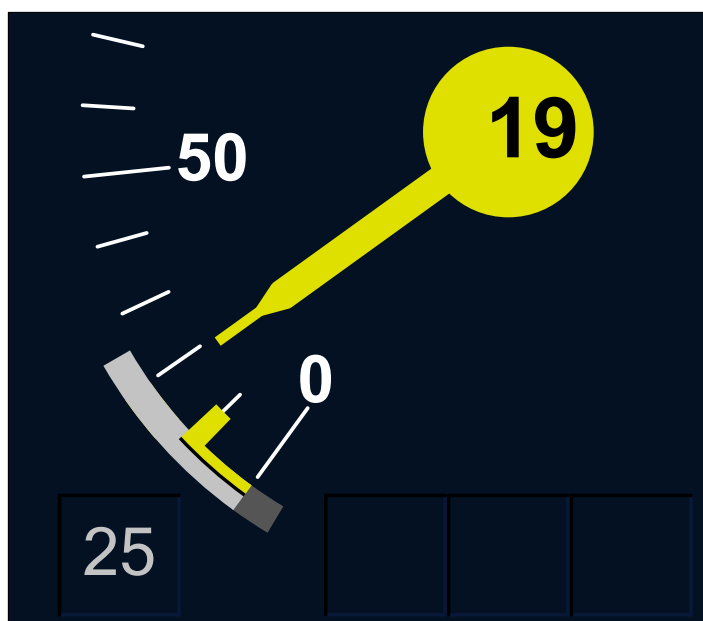
Figure 48 – Release speed, when V_{perm} < V_{release}
