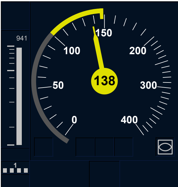
Figure 20 – Speed and supervision information in TSM / IndS (bubble 1c)
