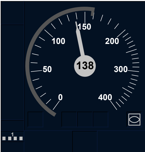
Figure 13 – Speed and supervision information in CSM / NoS (bubble 1a)
