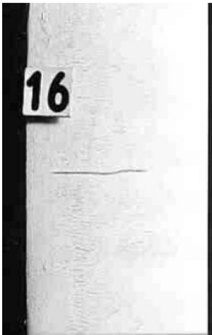
Transverse crack revealed by magnetic particle testing [EN 15313, §C.2.6 ]
