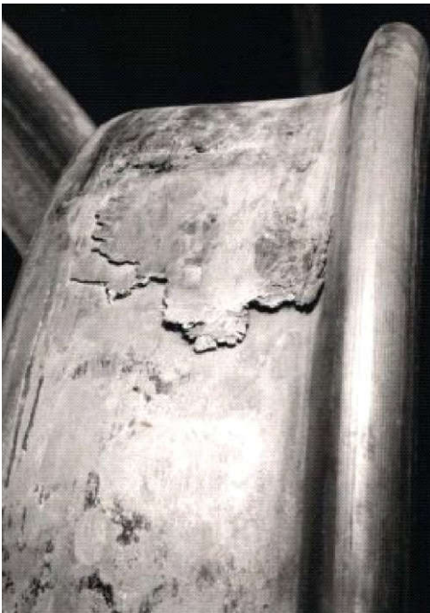
Metal build up on the tread
