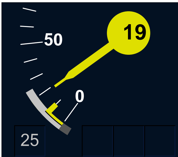
Figure 46 – Release speed, when V_{perm} < V_{release}
