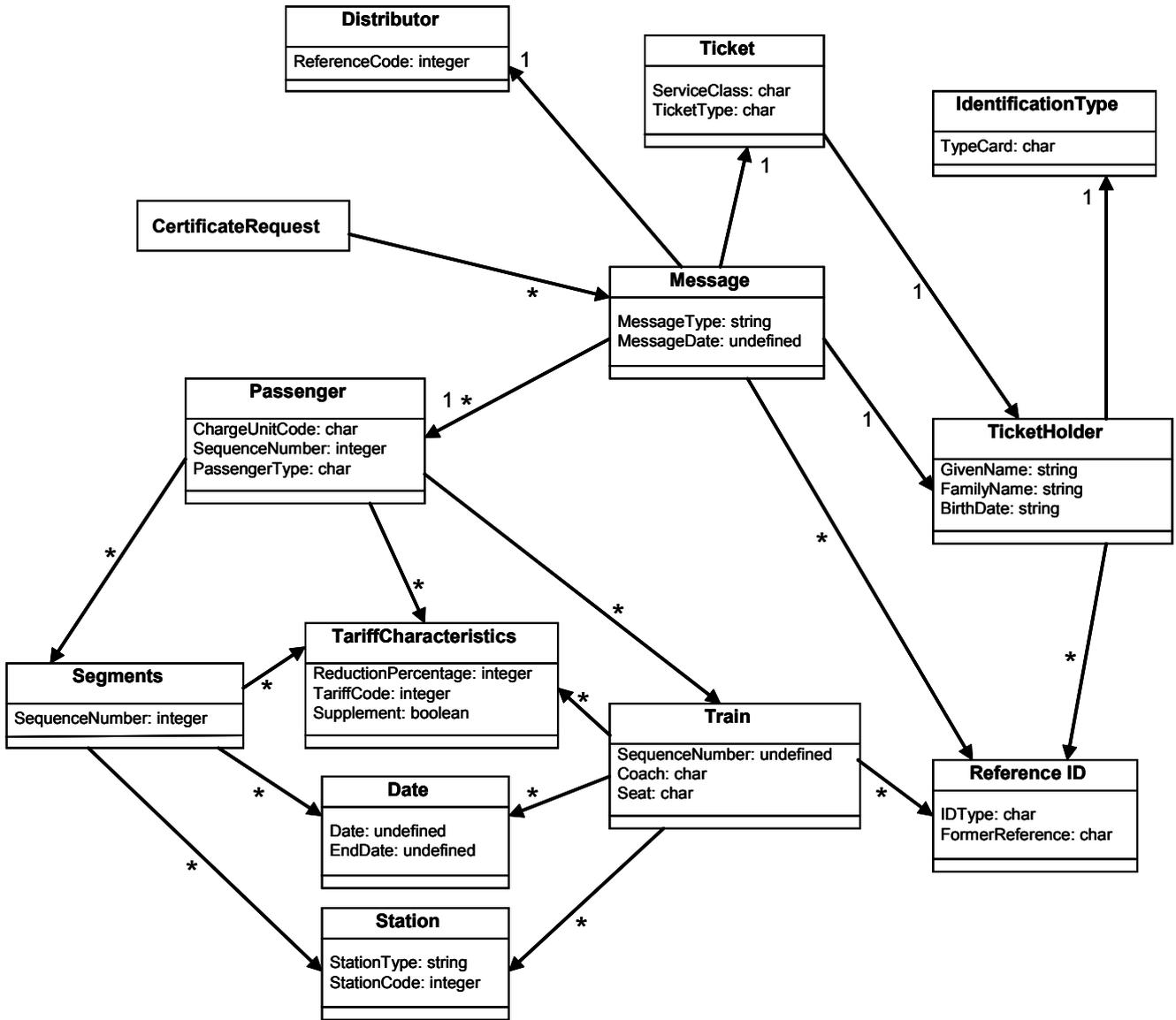
Fig.23 - Class diagram: Certificate Request\_Message
