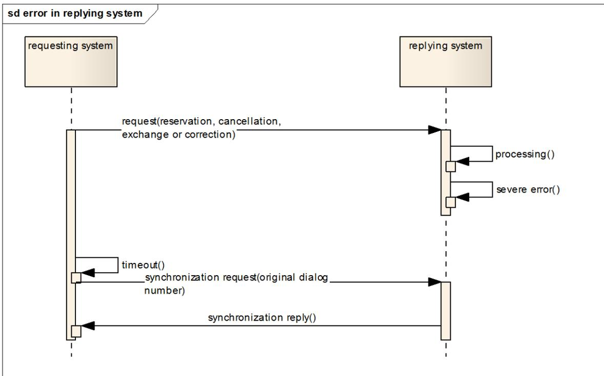
**A.2.3 - Defect before the reply is received from the replying system**
