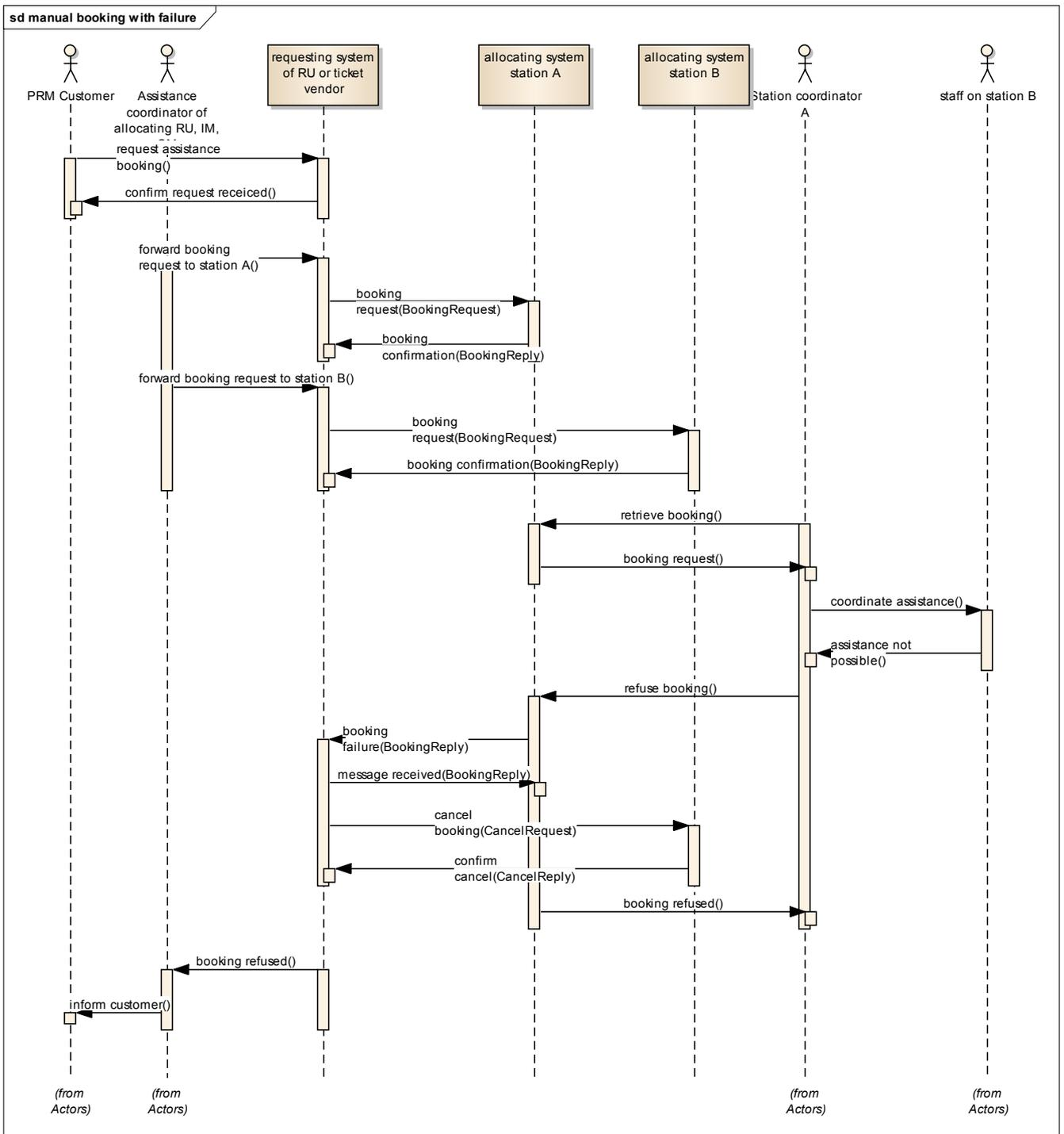
Figure 9 sequence diagram – manual booking with failure
