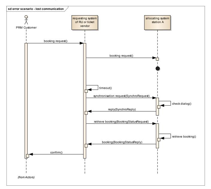
Figure 7 sequence diagram – error handling
