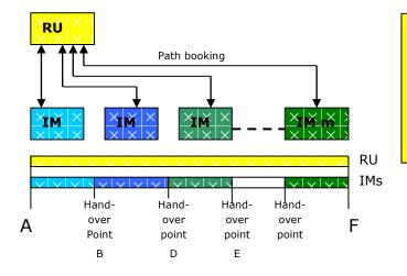
One RU is booking directly from the various IMs the several paths from A to F - section by section - between two handover points. The train must be operated by the RU for the complete journey, therefore no interchange points exist.
