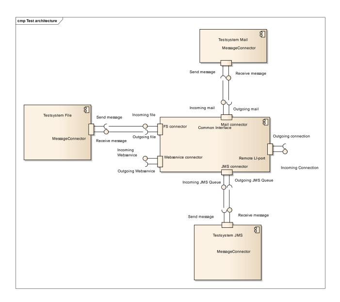
The test components for the connectors were realized by Mock-Ups written in Java. All tests were created as tests based on the test framework TestNG.
