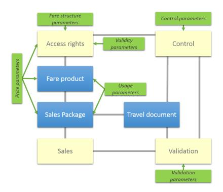
Figure 3 – Fare collection main processes and concepts (SCHEMATIC)
