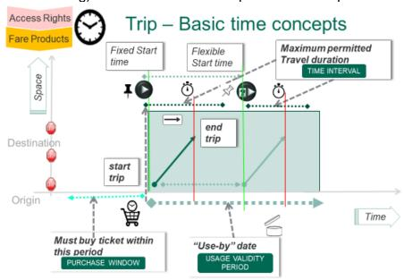
Figure 11 – Basic Time concepts for a single trip
