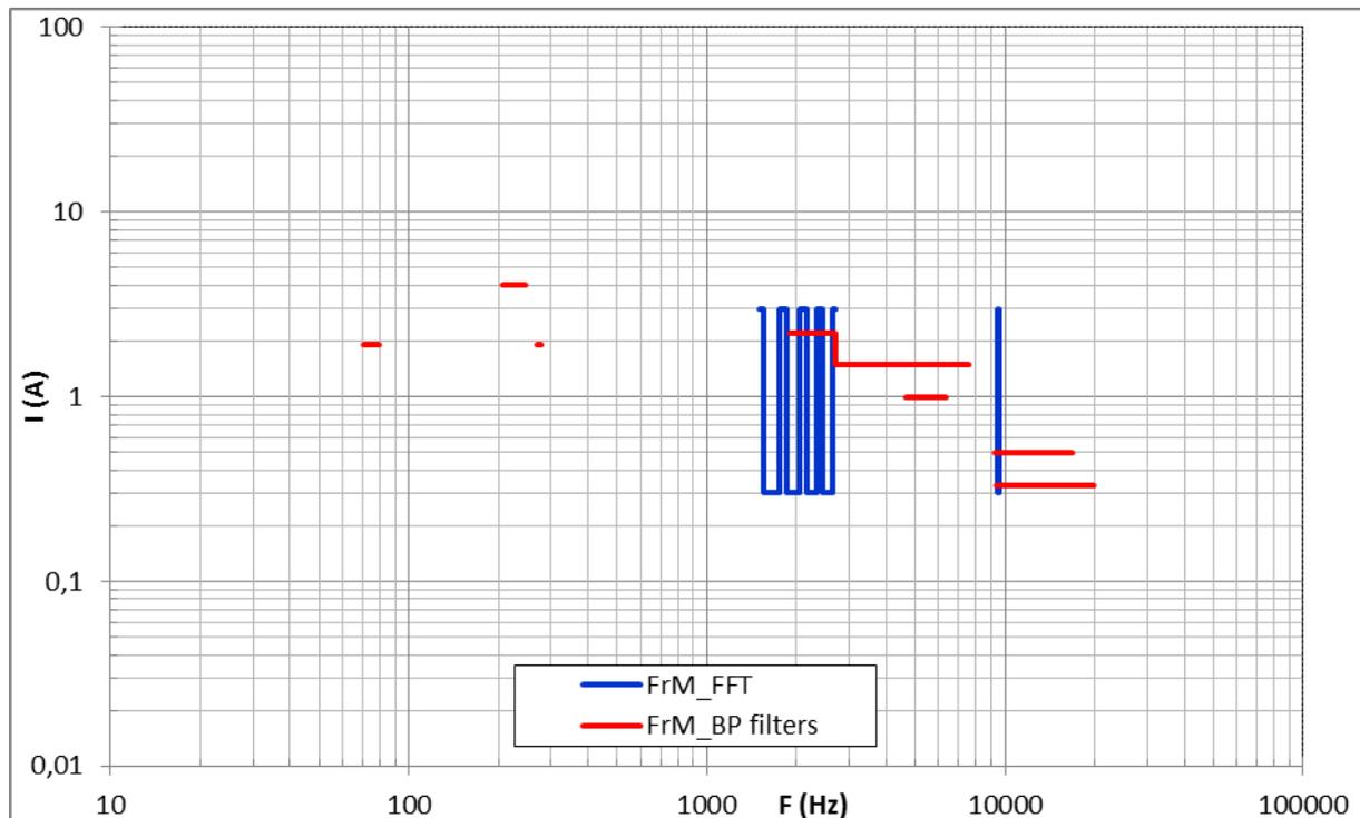
*Figure 15: Frequency Management DC traction*
