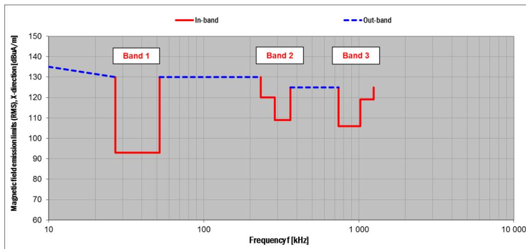
Figure 7: Compatibility requirements for X direction
