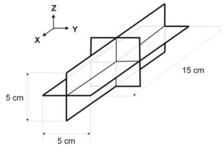
*Figure 11: Loop antenna*
