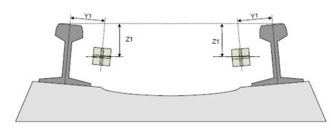
Figure 12: Position of the measurement antenna (internal between the rails)
