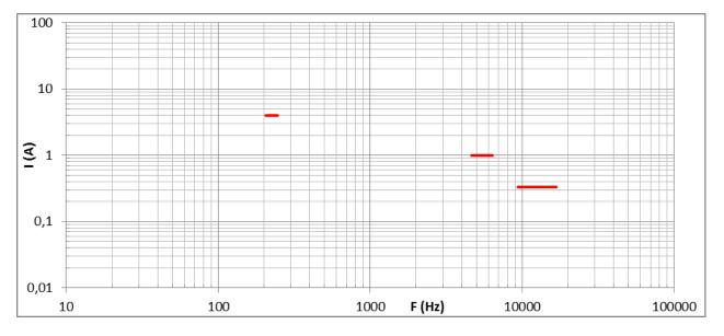
Figure 14: Frequency Management 15kV AC 16,7 Hz traction
