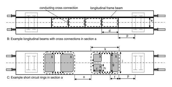
Resulting short circuit ring (electrically conducting loop)
