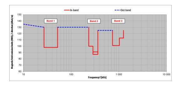
Figure 9: Compatibility requirements for Z direction
