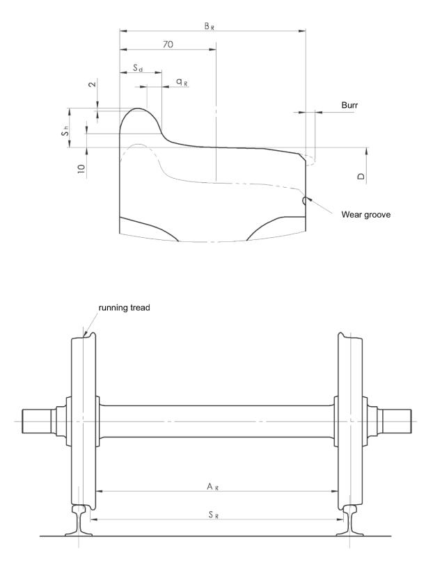
Figure 2: Wheel and wheelset dimensions
