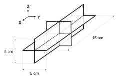
Figure 11: Loop antenna
