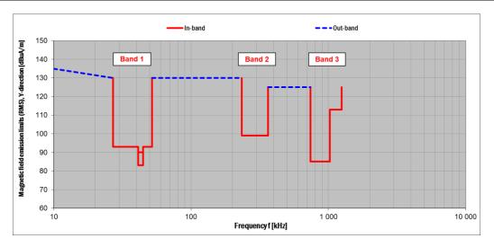
Figure 8: Compatibility requirements for Y direction
