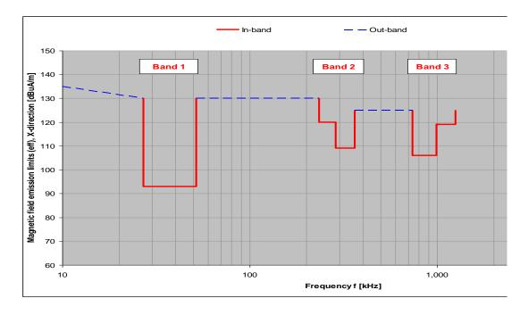
Figure 5: Compatibility requirements for X direction
