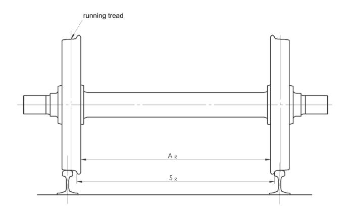
Figure 2: Wheel and wheelset dimensions
