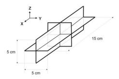
Figure 9: Loop antenna
