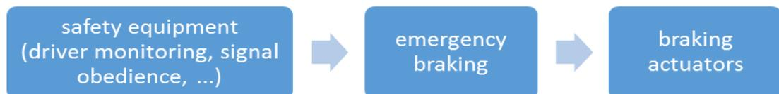
**Figure 20: Emergency braking functionality.**
