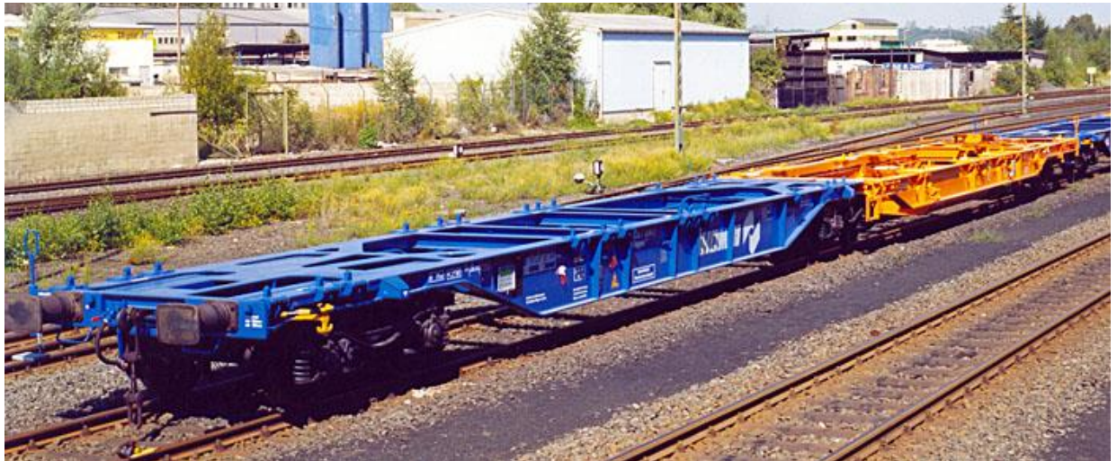
Figure 2: Example 1 of a unit consisting of a rake of permanently connected two elements (blue and orange), those elements cannot be operated separately (articulated wagon)
