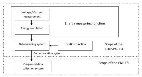
It is permissible to access the data in the EMS for other purposes (e.g. feedback to the driver regarding the efficient operation of the train) provided that it can be demonstrated that the integrity of EMS functions and data are not compromised by this arrangement.
