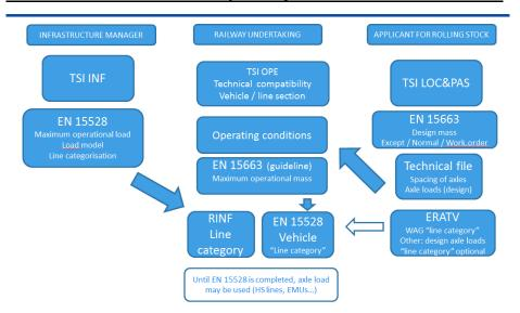
Fig. Principle of managing the axle load interface (when EN 15528 will be completed)
