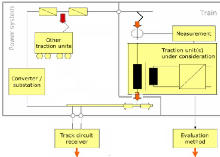
Figure 1.- Interference current flow (for track circuits)
