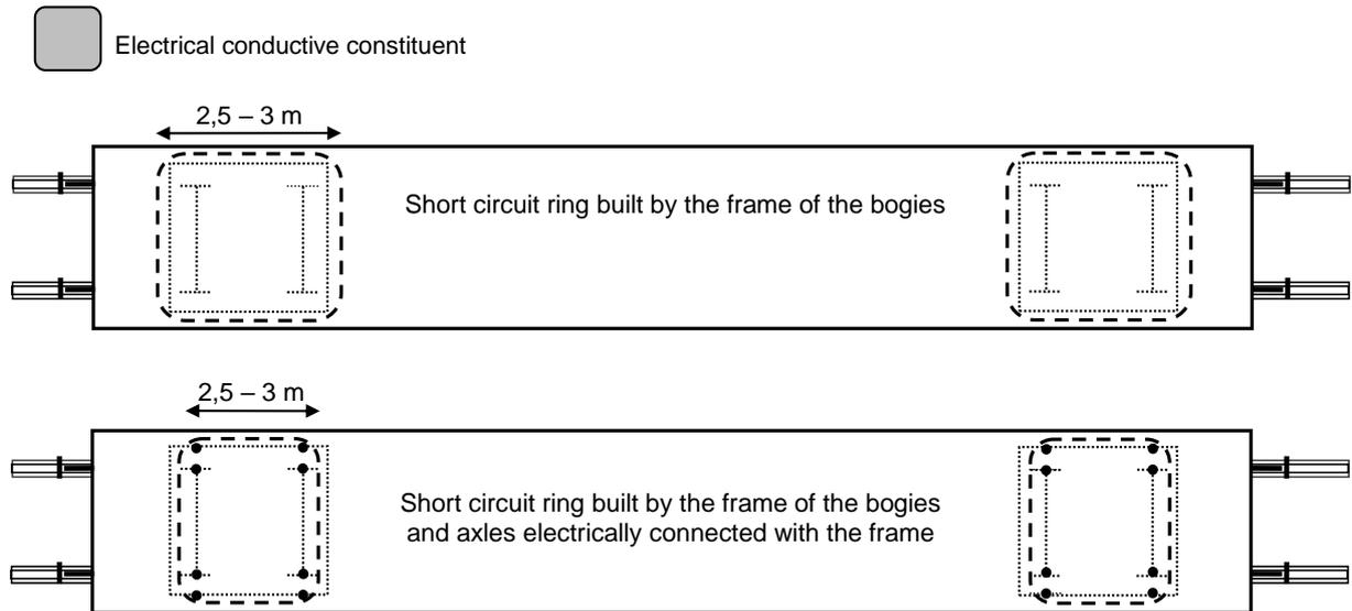
Figure 9.- Example for short circuit rings built by constructive and conducting parts of bogies with
