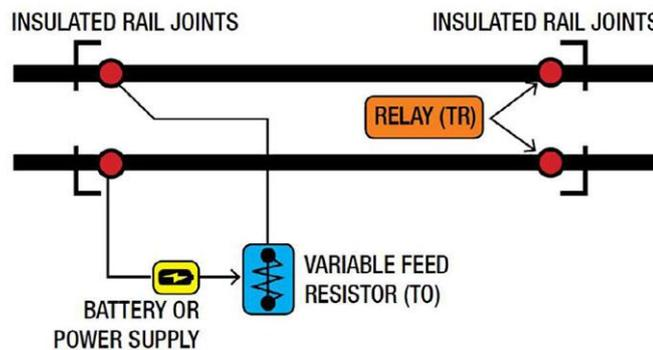
Figure 1.- Track circuit example
