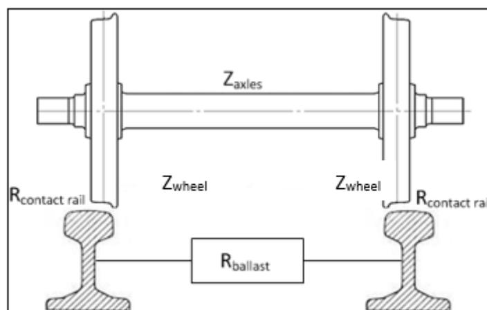
Figure 2.- Shunting impedance
