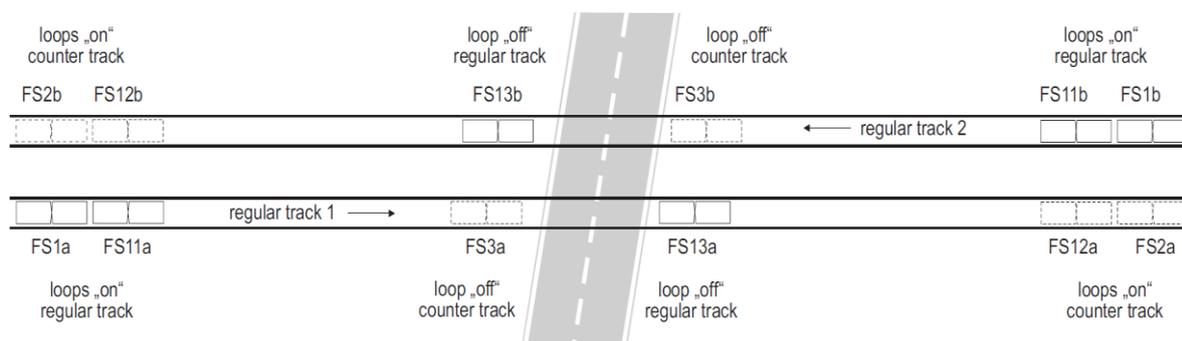
Figure 1.- Position of loops on level crossings - principle
