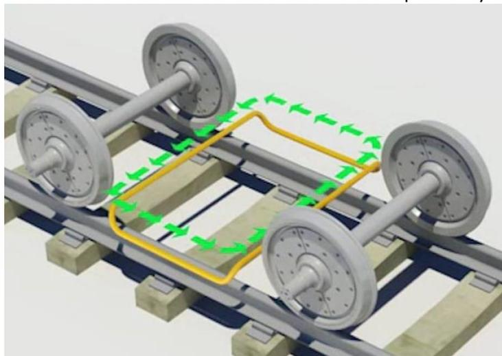
Figure 2.- Shunt assisting device – working principle
