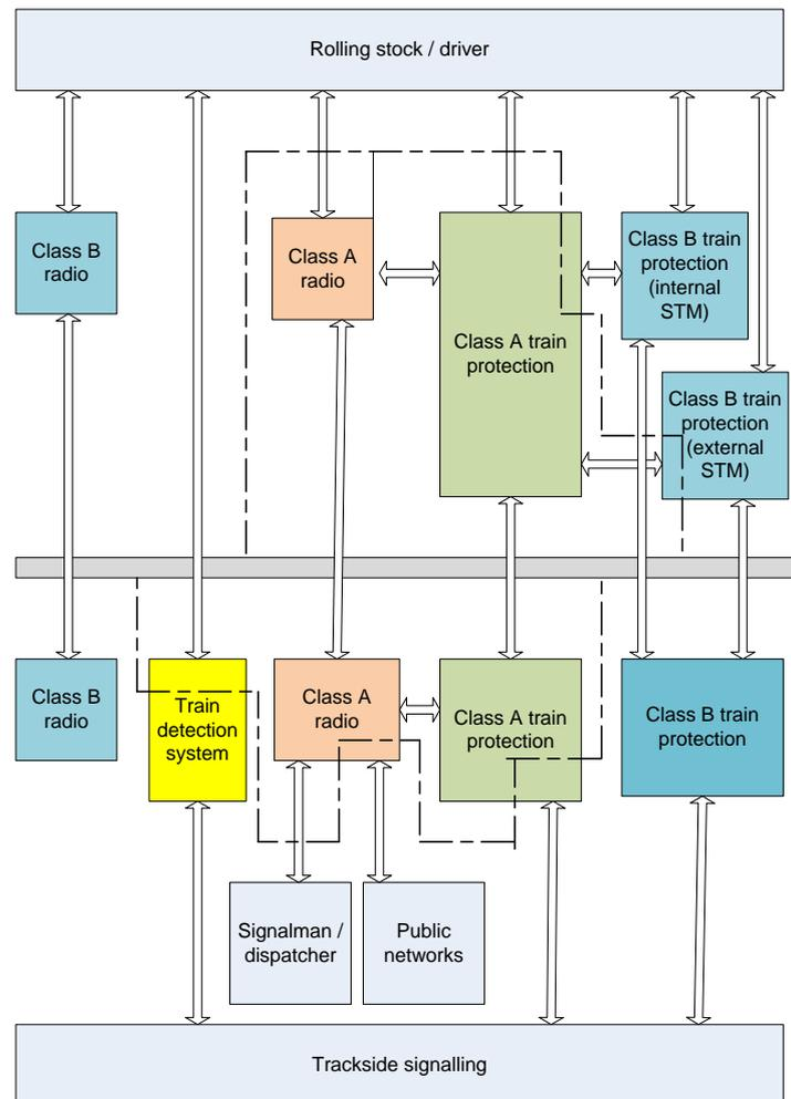
Figure 1: Scope of TSI Control-Command and Signalling
