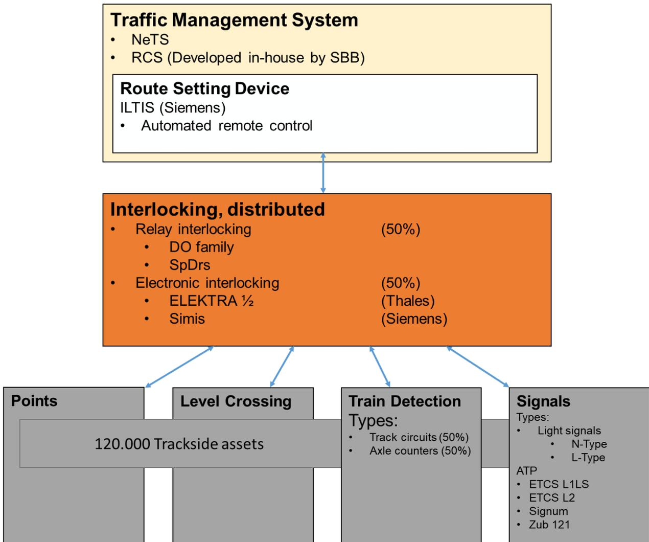
Figure 25: System architecture SBB
