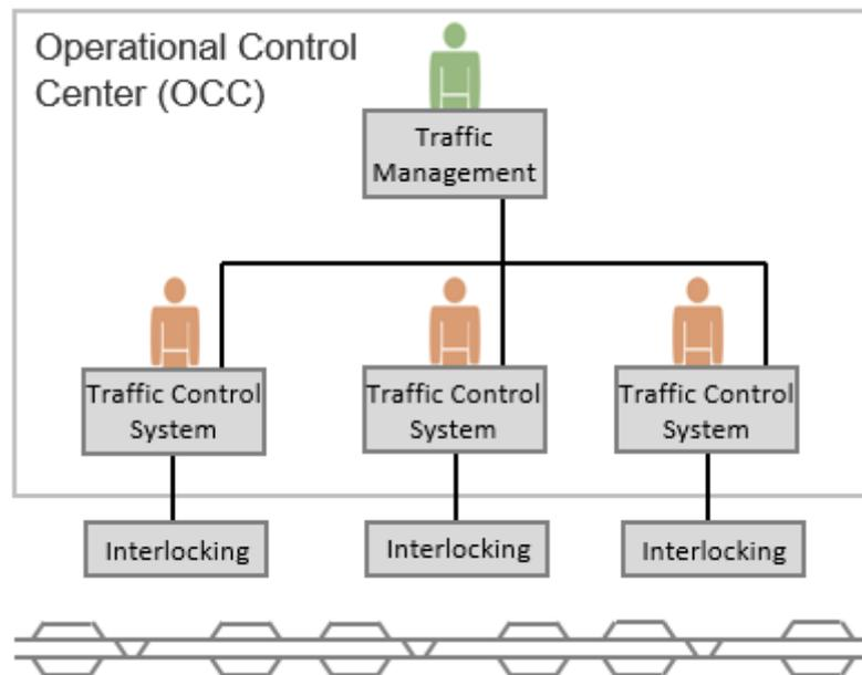
Figure 33: Centralised Traffic Control (CTC) with additional separated Traffic management.
