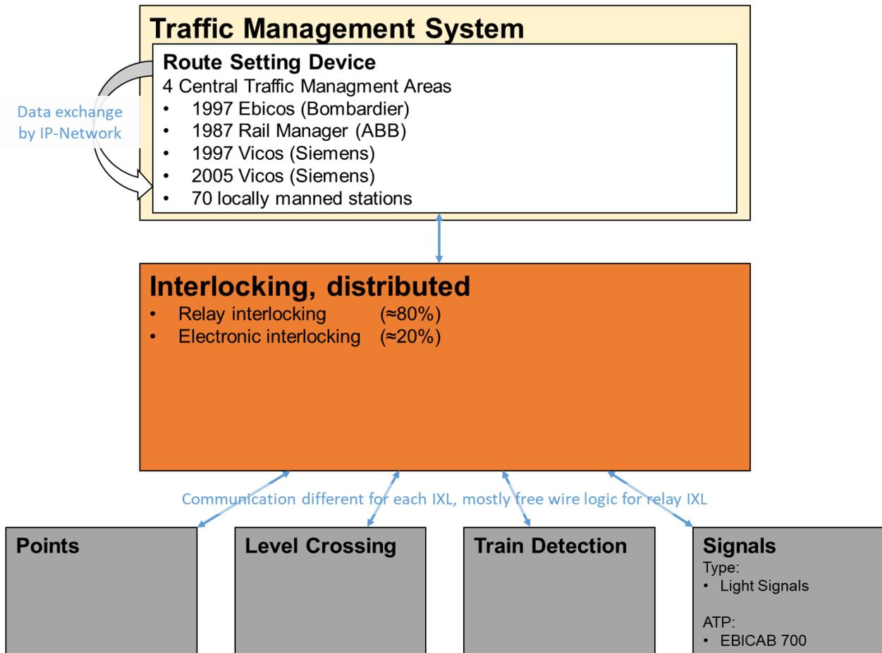
Figure 38: System architecture Bane NOR, [10.A].
