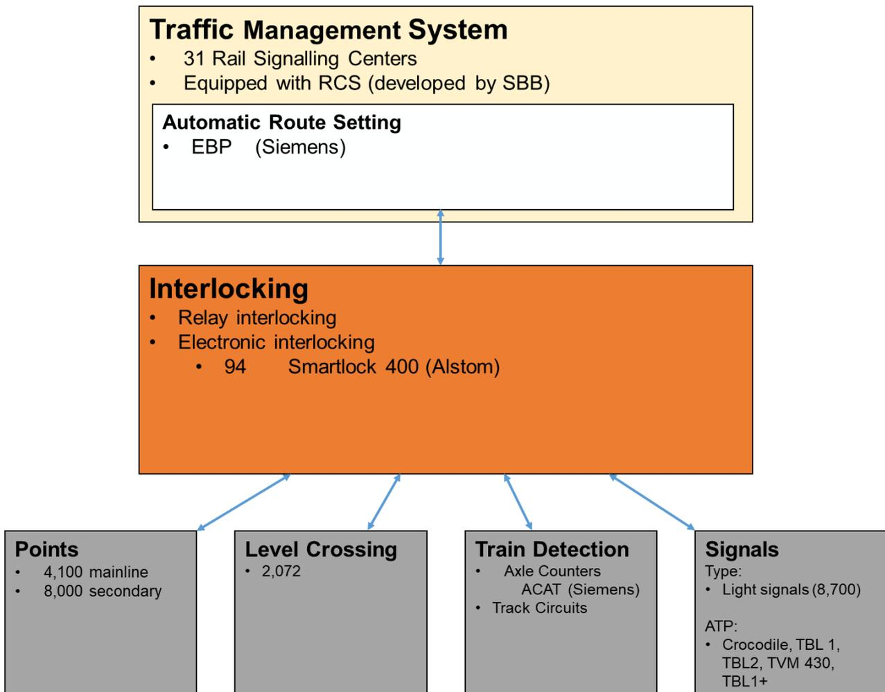
Figure 35: System architecture Infrabel. [8.B], [8.C]
