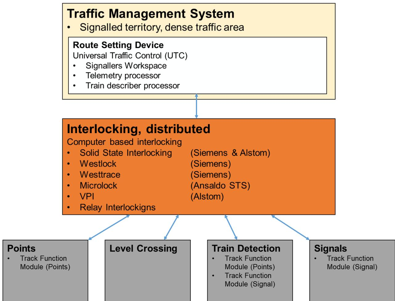
Figure 41: System architecture Queensland rail. [11.G], [11.H].
