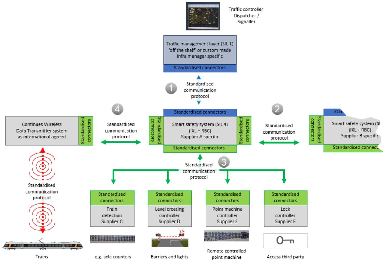
Figure 21. Reference optimum system architecture
