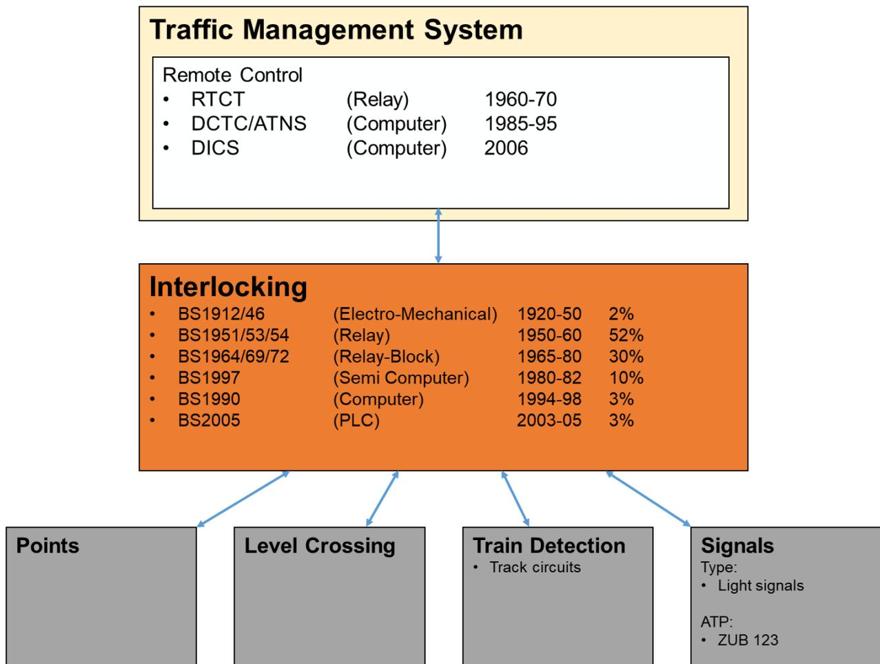
Figure 34: System architecture Banedanmark. [7.B], [7.C].
