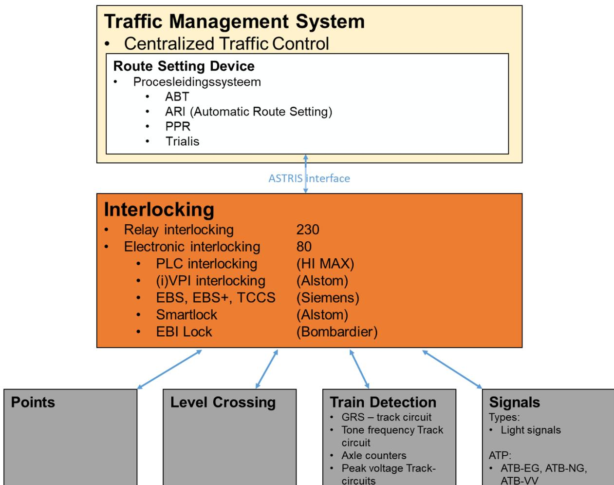
Figure 32: System architecture ProRail. [6.E]
