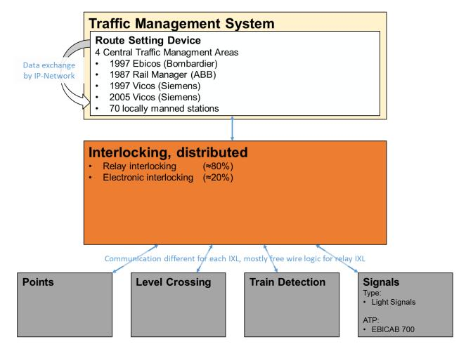
Figure 38: System architecture Bane NOR, [10.A].
