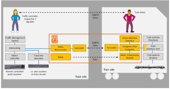
Figure 11: Simplified overview general system architecture ERTMS Level 2
