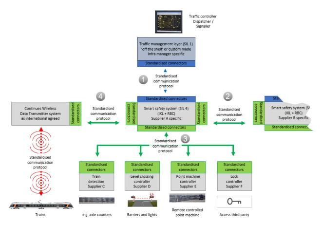
Figure 21. Reference optimum system architecture
