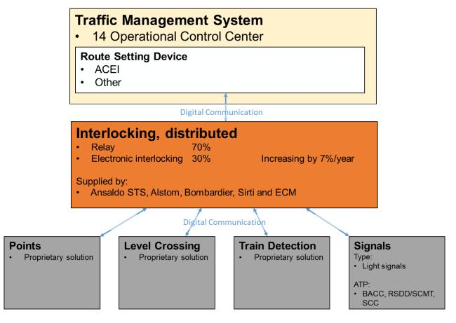
Figure 36: System architecture RFI [9.G]
