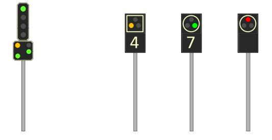
Figure 26: Simplified examples of the Swiss L (left) and N type signals (three on the right)
