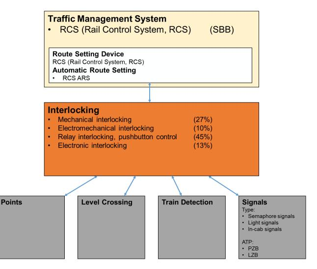
Figure 27: System architecture DB Netze [4.B], [4.D], [4.E], [4.F], [4.J].
