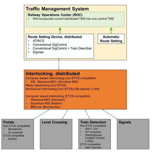
Figure 39: System architecture TfNSW. [11.D], [11.E], [11.F].
