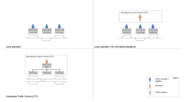
Figure 37: Types of traffic control centres maintained by the RFI.
