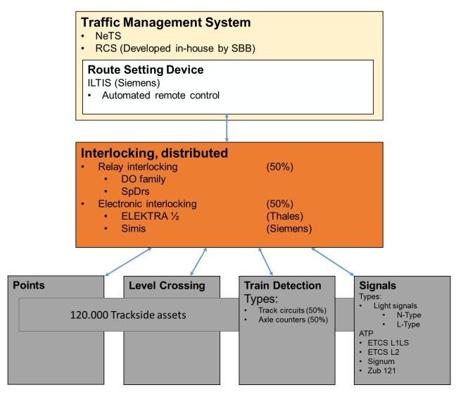
Figure 25: System architecture SBB
