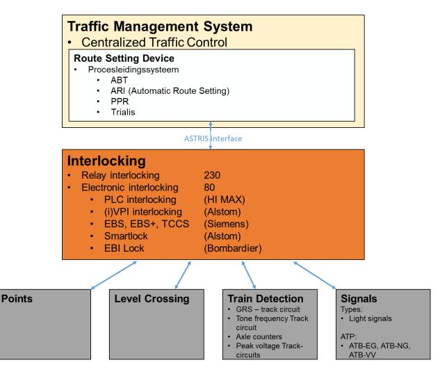
Figure 32: System architecture ProRail. [6.E]
