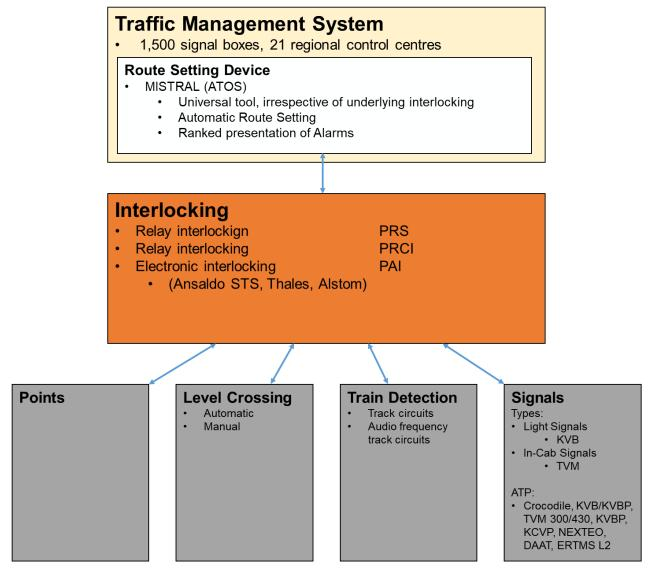
Figure 31: System architecture SNCF [5.A]
