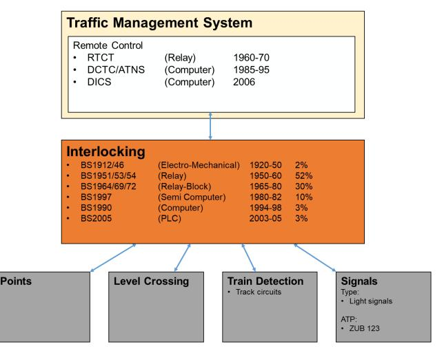
Figure 34: System architecture Banedanmark. [7.B], [7.C].
