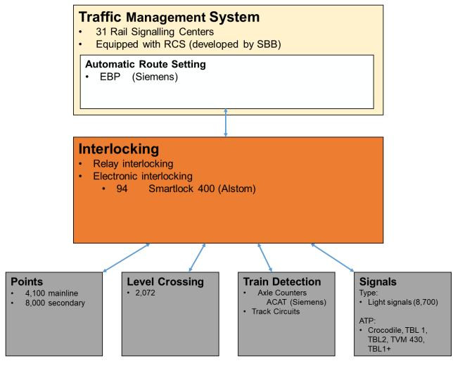
Figure 35: System architecture Infrabel. [8.B], [8.C]
