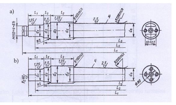
THE MAIN DIMENSIONS OF NEW WHEELSET AXLES, mm
