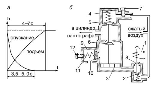
Pantograph valve: a – dependence of the contact skate lifting on time; b (δ) – pantograph valve arrangement
