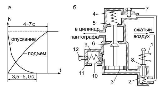
Pantograph valve: a – dependence of the contact skate lifting on time; b (6) – pantograph valve arrangement
