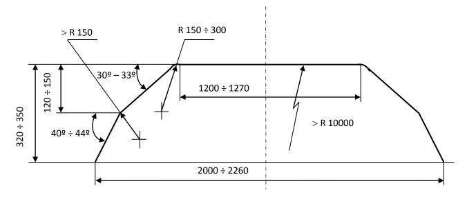
Fig. Configuration and dimensions of contact skates
