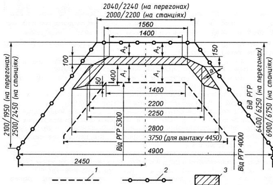
1 –clearance gauge of rolling stock; 2 – clearance gauge of artificial structures; 3 – position of the pantograph with regard to the shift thereof.
