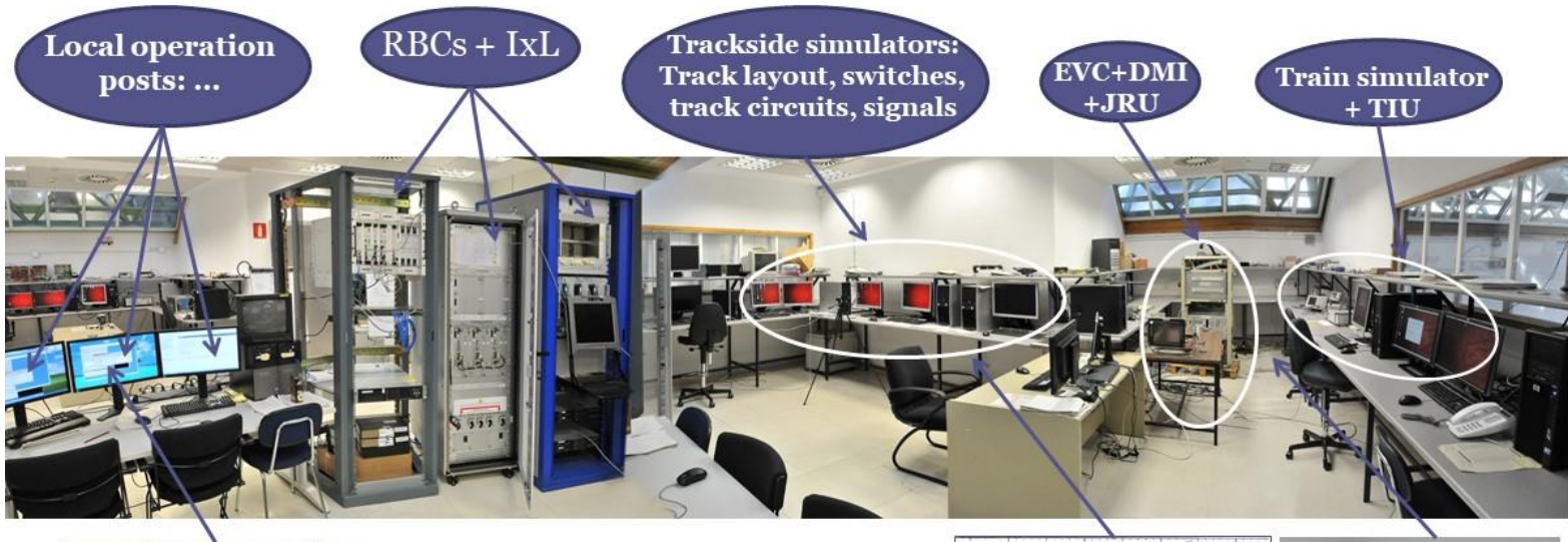
Panoramic view of a EAL: a ESC Test Campaign of a real line with two RBCs and one EVC
