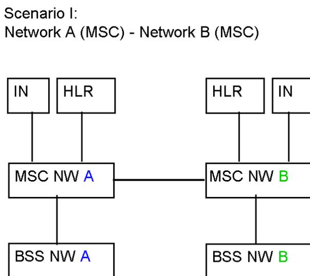
Figure 4.3: Test scenario I - Interconnection of two EIRENE networks
