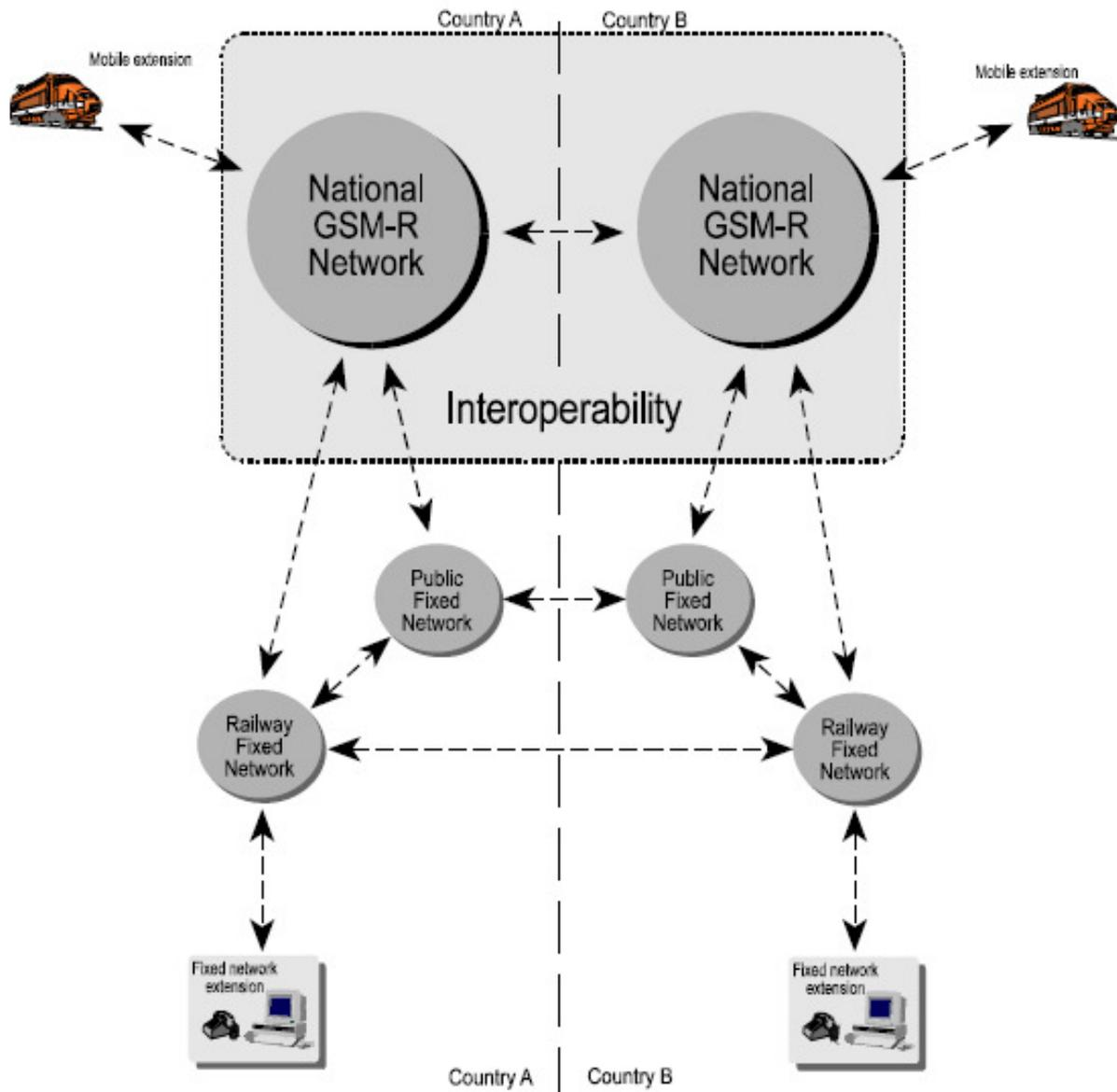
Figure 4.2: Overview of possible interconnections of EIRENE and non EIRENE networks (source: UIC, Draft GSM-R Procurement & Implementation Guide)
