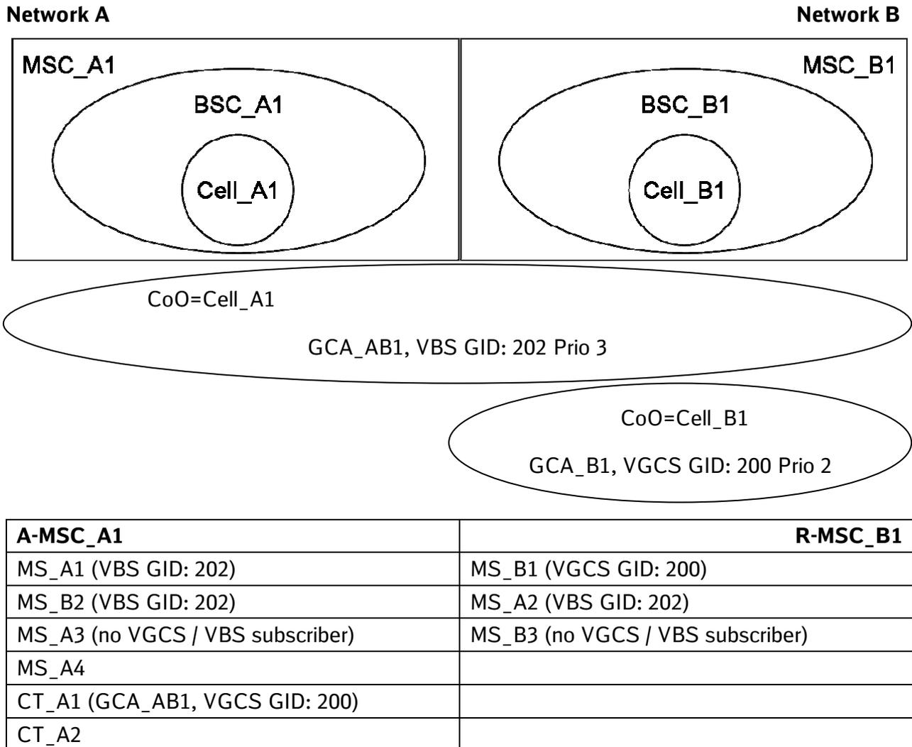
Figure 4.6: Example description of test configuration used in the IOT test specification
