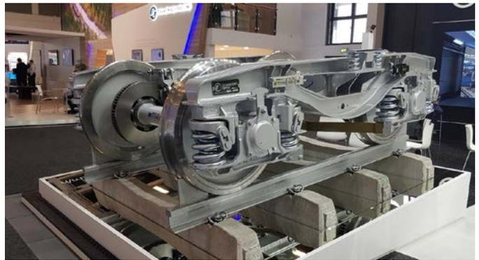
**ABOVE:** Two silent wagon bogies fitted with disc brakes
