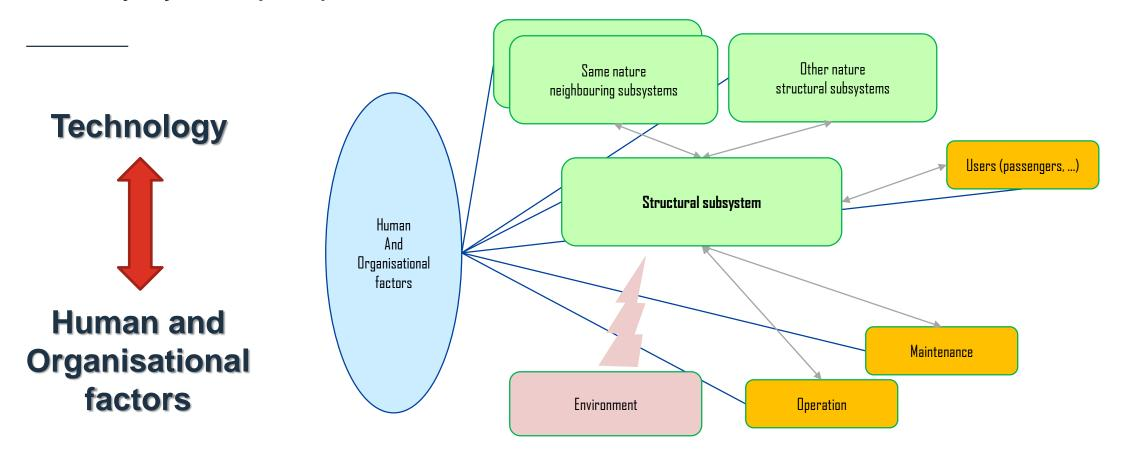
A system comprises not only its technical components but also the interaction with the humans developing, operating, and maintaining it
