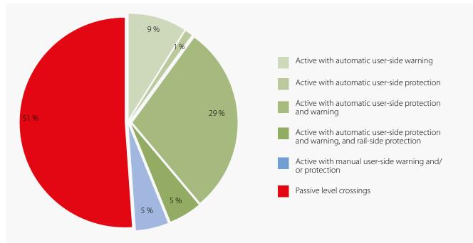
Figure 20: Breakdown of level crossings according to type in 2012 (EU-28)
