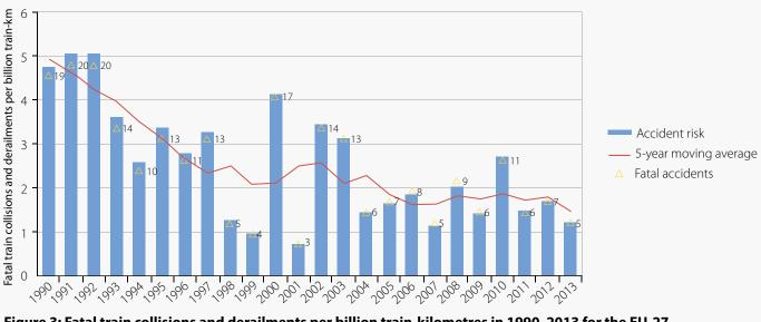
Figure 3: Fatal train collisions and derailments per billion train-kilometres in 1990–2013 for the EU-27, Switzerland and Norway (<sup>4</sup>)
