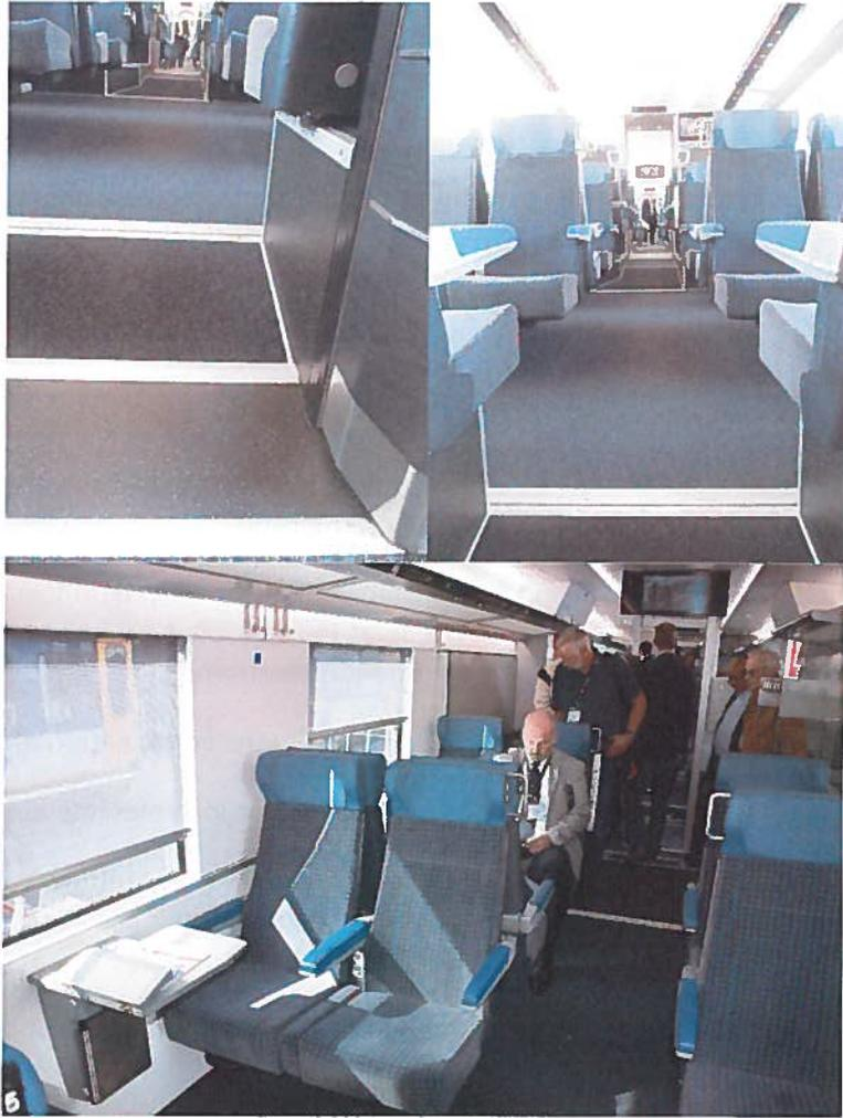
Figure 15. The internal ramp, interior floor levels and general internal layout. (©Antoine Defosseze/ERA and David Haydock)
