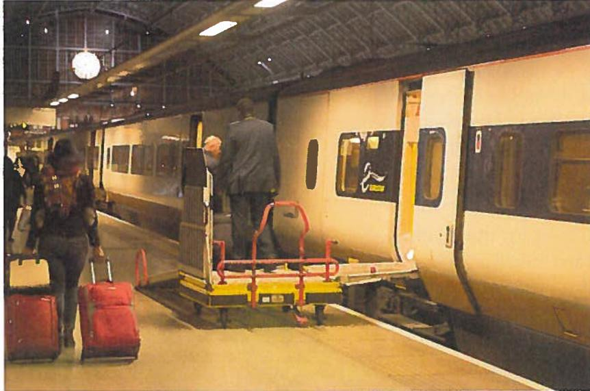
*Figure 8. HS1 boarding aid being prepared for use on EIL Class 373 train at London St Pancras station. Platform height complies with the TSI 760 mm arl target. (© ERA/Ernest Godward)*
