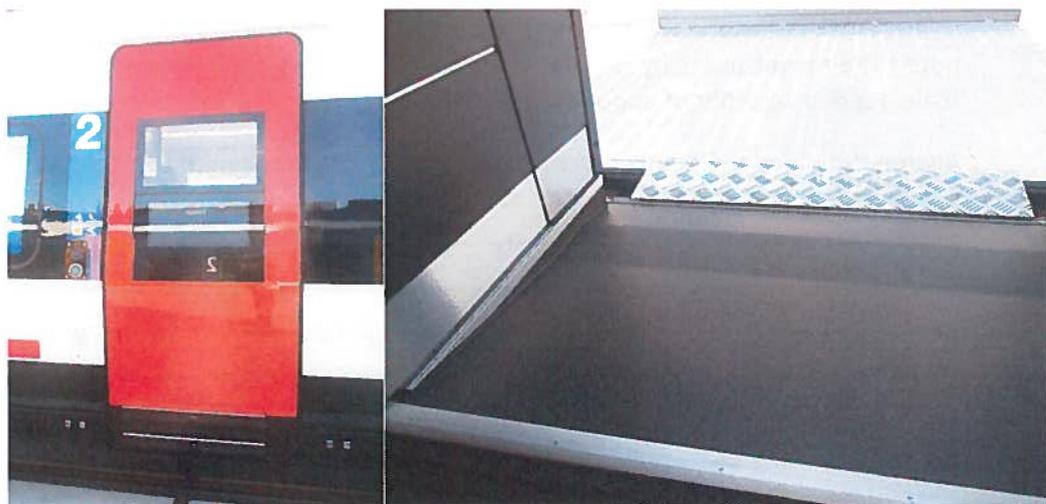
Figure 14. The new Stadler HST for SBB with level boarding to ramped internal access. (©Antoine Defossez/ERA)
