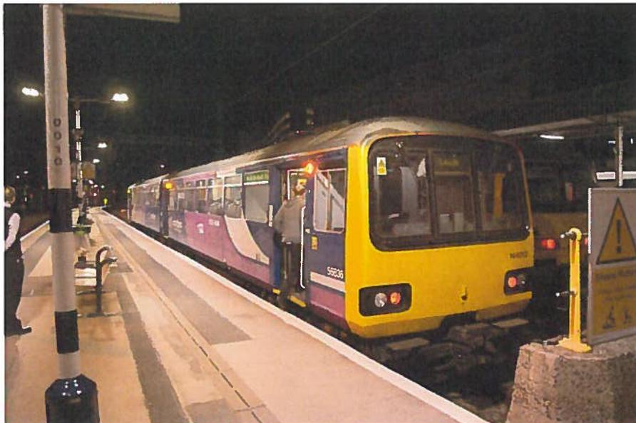
Figure 4. UK typical “one step boarding” from specific case platform height 915 mm arl observed at Doncaster railway station (© ERA/Ernest Godward)
