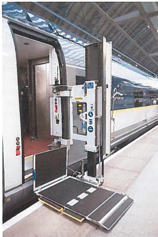
*Figure 9. EIL Class 374 train boarding aid in the deployed position at London St Pancras station – platform height 760 mm arl. (Courtesy and ©Eurostar International Limited)*
