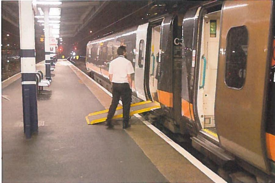
Figure 5. UK PRM boarding ramp from specific case platform height 915 mm arl observed at Doncaster railway station (© ERA/Ernest Godward)
