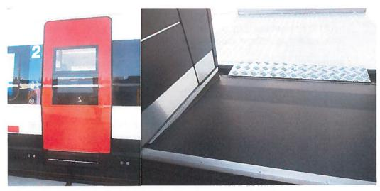
Figure 14.The new Stadler HST for SBB with level boarding to ramped internal access. (@Antoine Defossez/ERA)
