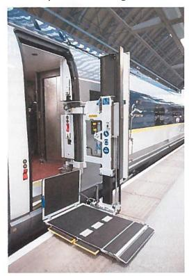
Figure 9. EIL Class 374 train boarding aid in the deployed position at London St Pancras station – platform height 760 mm arl.
