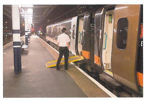
Figure 5. UK PRM boarding ramp from specific case platform height 915 mm arl observed at Doncaster railway station (© ERA/Ernest Godward)
