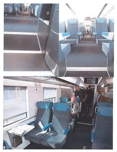
Figure 15.The internal ramp, interior floor levels and general internal layout. (©Antoine Defossez/ERA and David Haydock)
