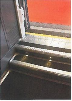
Figure 10 left. Current fixed steps (© ERA/Ernest Godward) for access to Alstom Duplex trains at platform heights of 550mm arl.
