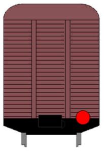
The reflective disc shall have a diameter of 185 mm with a red circle diameter of 140 mm.
