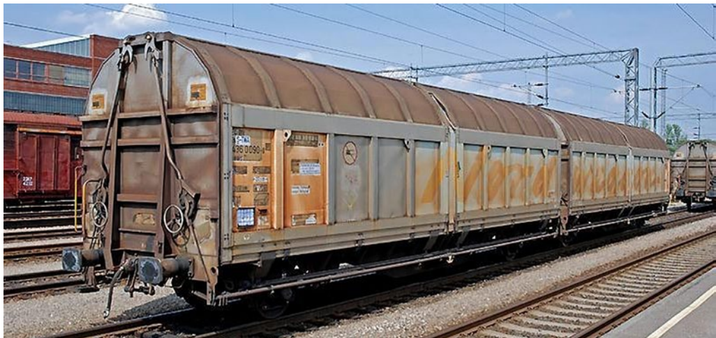
Picture 3: Example of a unit consisting of a rake of permanently connected two elements, those elements cannot be operated separately
