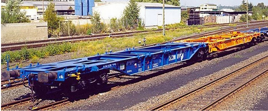
Picture 3: Example of a unit consisting of a rake of permanently connected two elements, those elements cannot be operated separately
