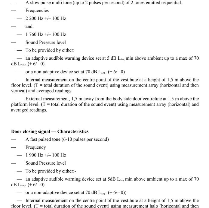
— External measurement, 1,5 m away from the body side door centreline at 1,5 m above the platform level. (T = total duration of the sound event) using measurement halo (horizontal) and averaged readings.
