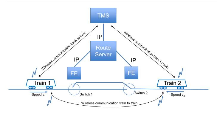
Figure 5 – Architecture of a future Command and Control 4.0 system. Smart wayside objects (field elements, FE) have open interfaces and powerful degraded modes. On the train, clearly only one interface is necessary, the communication interface between the rail vehicle and the external world.
