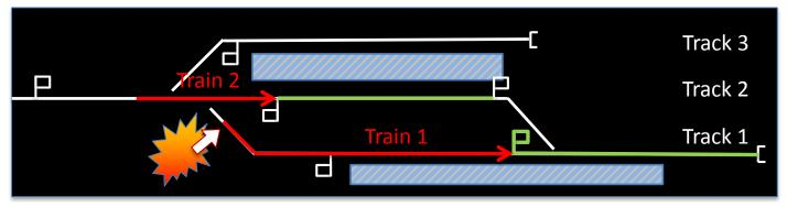
Train 2 is entering the station towards Track 2, and hits the rear end of Train 1. At the same moment, the signal on Track 1 is opened to enable Train 1 to use the entire platform
