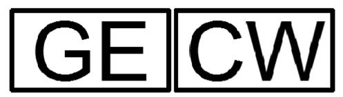
The letters shall be of the same font type as the TEN marking. The size of the letters shall be at least 100 mm high. The outer measures of the frame shall be at least 275 mm wide and 140 mm high, the frame shall be 7 mm thick.
