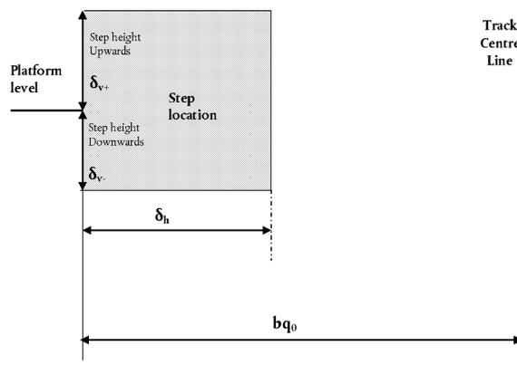
(2) The values of  $b_{q_0}$ ,  $\delta_h$ ,  $\delta_{v+}$  and  $\delta_{v-}$  depend on the type of platform where the rolling stock is intended to stop. They shall be as follows:
