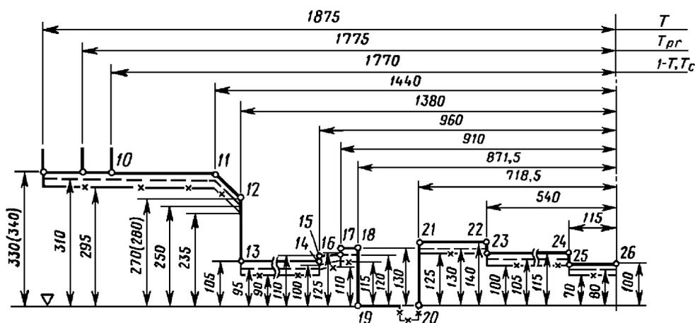
Note: For the rolling stock which is intend to be used on track of 1520 mm, able to pass over marshalling humps and rail brakes.
