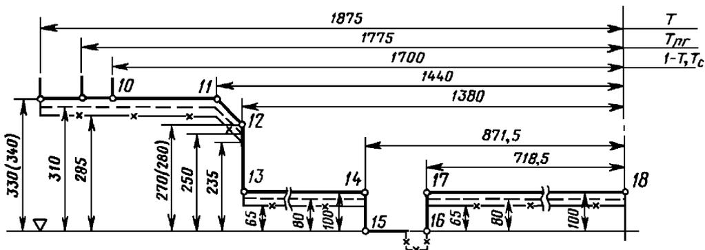
Note: For the rolling stock which is intend to be used on track of 1520 mm, with the exception to pass over of marshalling humps equipped with rail brakes.
