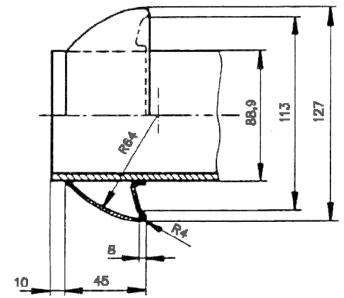
Quick connector SFS 4428, connector part A, size DN80
