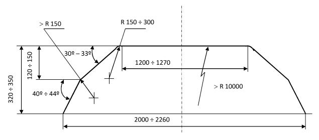
Fig. Configuration and dimensions of contact skates
