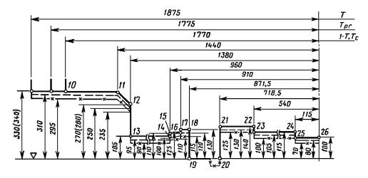
*Note:* For the rolling stock which is intend to be used on track of 1520 mm, able to pass over marshalling humps and rail brakes.
