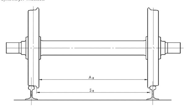
4.2.3.5.2.2 Mechanical and geometrical characteristics of wheels
