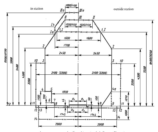
••••• zone where structures may be allowed (e.g. signals, ballast profile, etc.)
