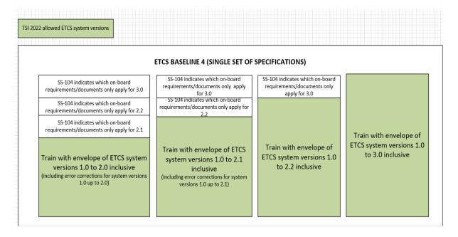
The enhancements which justify a new envelope of ETCS system versions 2.2 and 3.0 are elaborated in section 5.2.15 of this report.
