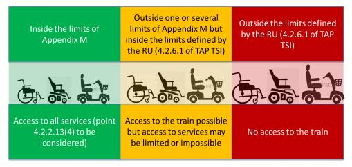
Figure 1: accessibility of wheelchairs according to their dimensions
