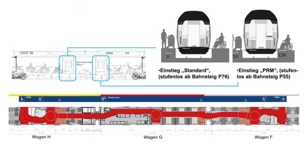
Figure 2 – Example of rolling stock giving level access from platforms at 550mm and 760mm and permitting circulation throughout to the adjacent car
