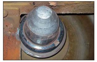
axles (32 and 33) of the wagon occupying the fourteenth place in the train set in the direction of travel were derailed and the second wagon axle had lost its right-hand axle box.
