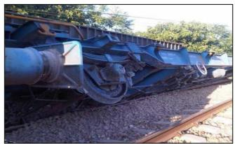
located in the Auxiliary Control Centre of Cordoba, due to overheating (151°C) in the axle box on the left-hand side of axle 39 in the direction of travel. When the head of CTC [Centralised Traffic Control] of the Cordoba Control Centre became aware of the alarm, he unsuccessfully tried to contact the driver of train CGX10 via the analogue (trainground) radio-telephone system, to inform him that the axle was overheating.
